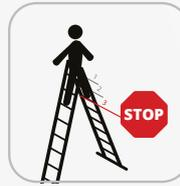
The top two steps or rungs of an A-frame ladder must not be used for standing, with the exception of podium ladders or other platforms specifically built for standing.
