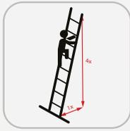
Before climbing, always make sure the ladder is placed in the correct position.
