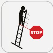
The top three steps or rungs of a leaning ladder must not be used for standing. This ensures that the ladder will provide maximum support and stability.
