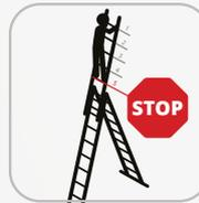
When climbing a combination ladder in freestanding position, the top four steps or rungs of the extension part must not be used for standing.
